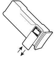
pack. The orientation of the battery contacts is shown in a picture on the inside bottom of the 9V battery compartment. Replace the 9V battery compartment door by reversing the process used to remove the door.
