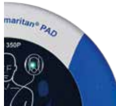
Figure 10. Flashing green LED; no action required.
