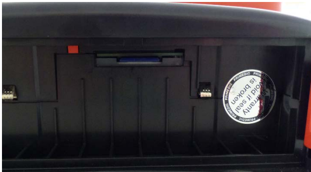
Fig. 13: Inserting / replacing the SD-card
